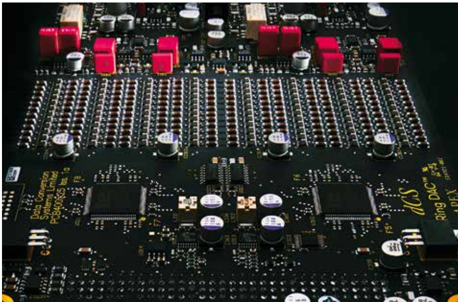
ABOVE: Overview of the latest APEX PCB with one Xilinx DSP [bottom] and matrix of 48 resistor current sources [centre] per channel, and analogue output stages [top, into distance]
