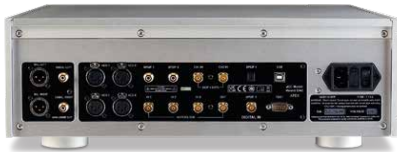
ABOVE: Four S/PDIF inputs (one optical and three coaxial) are offered alongside four AES/EBU inputs (or two pairs), one asynchronous USB (to 384kHz/24-bit PCM, DSD128 in DoP), three Word-Clock inputs/one output (on BNCs) and both single-ended (RCA) and balanced (XLR) fixed/variable audio outputs
